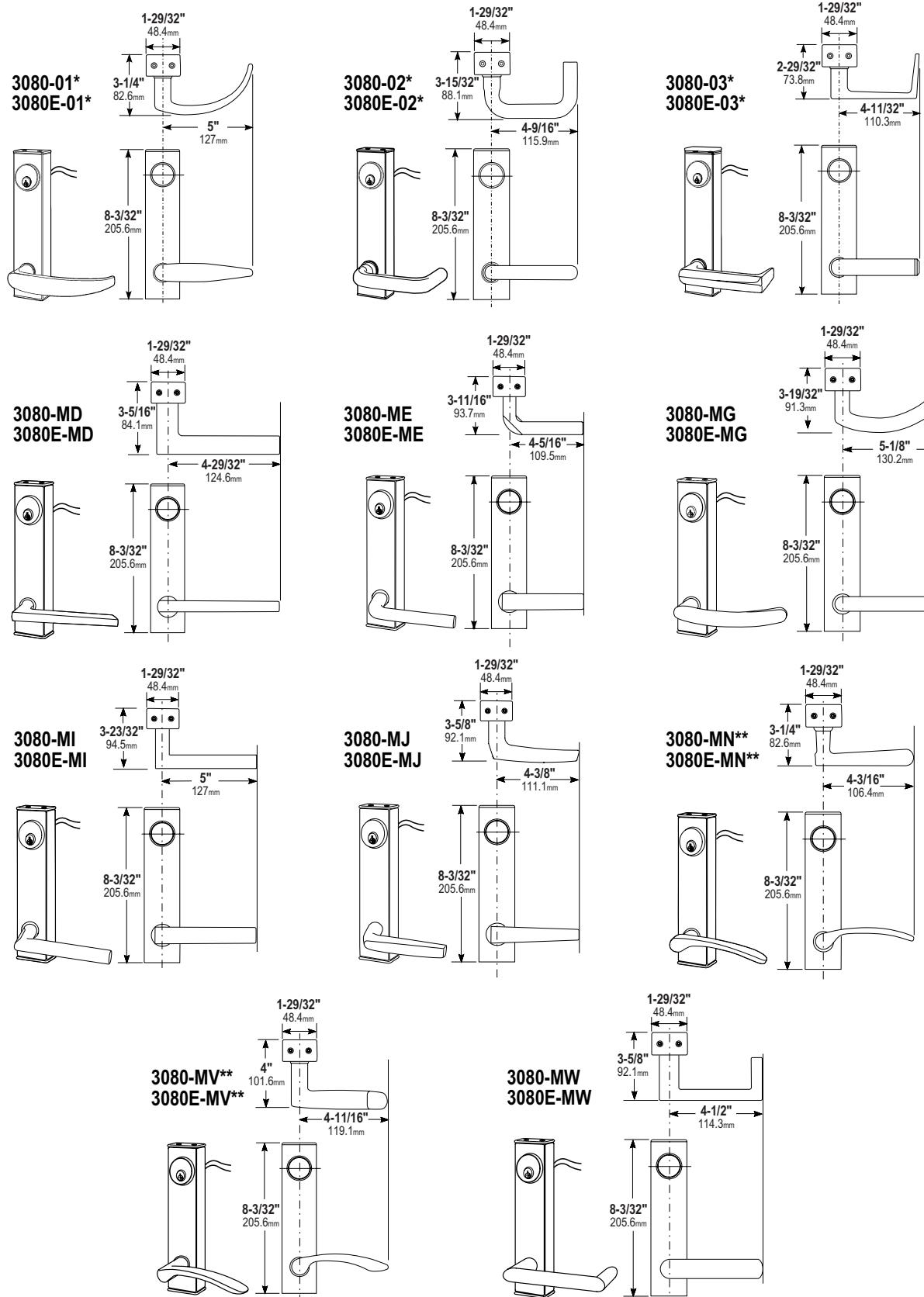
\* The 3080-01, -02, and -03 lever handles are designed to return within 1/2" of the door face. Handles in the Designer Series do not have this same feature. Please verify with local code requirements to ensure compliance.
