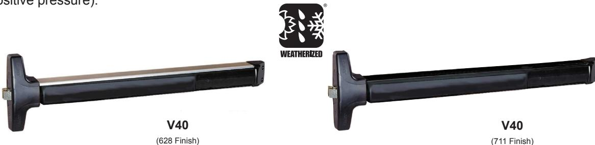
Standard V40 Rim Device accommodates wide stile doors, 3" or greater stile, and flush doors. For Narrow Stile doors, 2" to 2 1/2" stiles, specify V40 NS model which provides a 2" longer device and a lower profile strike.
