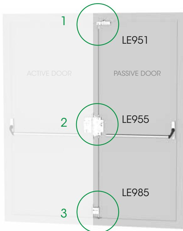
**PE928** Passive door leaf products for wooden or metal doors (incl. LE951, LE955, LE985) are ordered by product code PE928.
